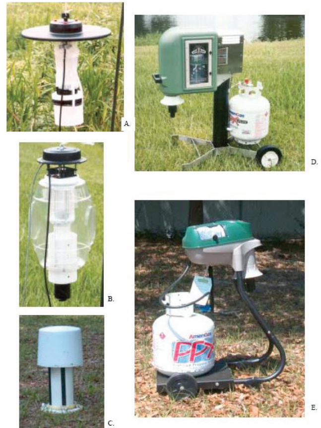
Figure 2: Five mosquito traps evaluated at the University of Florida Horse Teaching Unit: A. CDC-1012; B. Mosquito Magnet-X; C. Home and Garden Mosquito prototype trap; D. Mosquito Magnet Pro; E. Mosquito Magnet Liberty.
